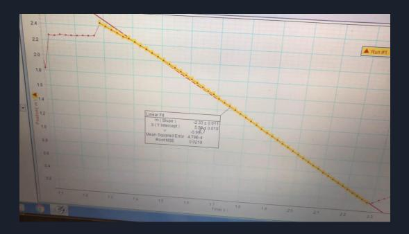
Students were asked to predict the velocity of the cart when it reached the bottom of the incline. The graph students created using Data Studio was a distance time graph. By using the linear fit tool and selecting the proper part of the graph the students were able to find the slope of the graph which represents the final velocity of the cart.
